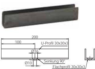
Tripod attachment for two lamps: Item 045187
