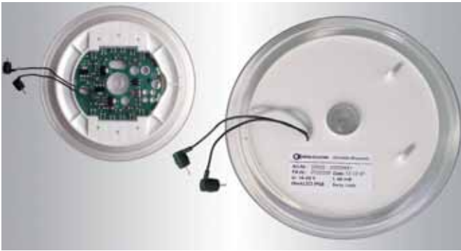
Electronic sealed with sealing compound
