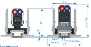
view: cut of the profile with current collector
